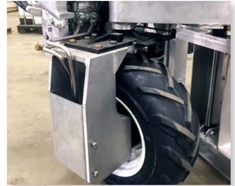
The parking brake interrupts the flow of hydraulic fluid to the orbital motor and locks the drive wheel in place. The parking brake should be used when connecting the dolly to a tank and for transporting on a utility trailer.
